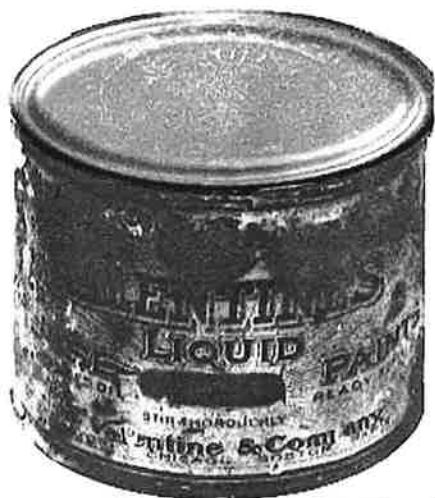
Photo of a hand-soldered can of paint from the 1880's. The company claims that the paint inside is still usable.
